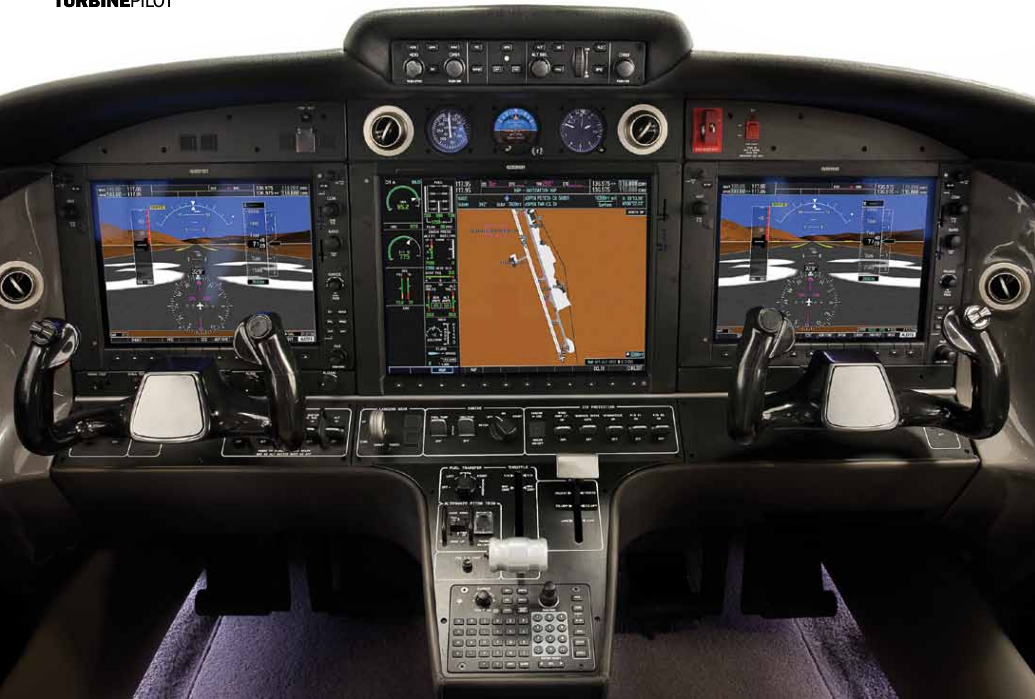
A mockup of the D-Jet's panel (left) features the Garmin G1000 avionics suite and a glareshield-mounted GFC 700 autopilot/flight control system. A keypad beneath the thrust lever is used to make entries on the G1000. Lighting and temperature controls are on an overhead panel (above). Diamond came up with a clever design for the two-piece airstair door, in development when this story was written (below). When the door opens, a panel deploys to both shield the engine inlet and provide a passenger handrail.
