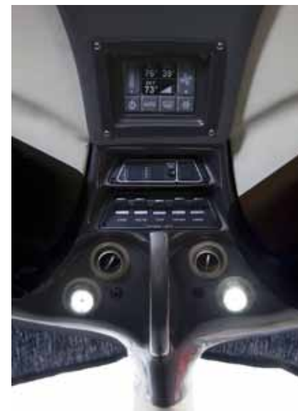
A mockup of the D-Jet's panel (left) features the Garmin G1000 avionics suite and a glareshield-mounted GFC 700 autopilot/flight control system. A keypad beneath the thrust lever is used to make entries on the G1000. Lighting and temperature controls are on an overhead panel (above). Diamond came up with a clever design for the two-piece airstair door, in development when this story was written (below). When the door opens, a panel deploys to both shield the engine inlet and provide a passenger handrail.
