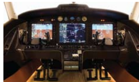
The D-JET's well-appointed flight deck is centered around a three-screen Garmin G1000 system
