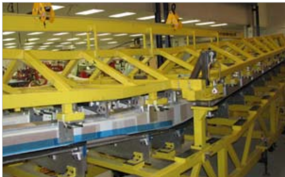
When the tooling is opened, a finished wing will emerge.
