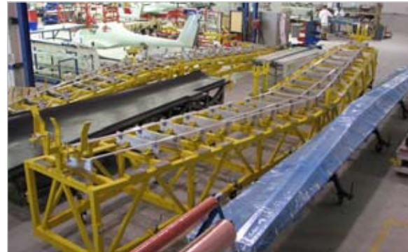
Sophisticated wing assembly fixtures ensures precise positioning of spars, ribs, wing skins and attachment fittings.
