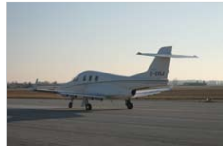
D-JET S/N 001 taxiing out to test the new ventral strakes, which will be part of the production configuration.
